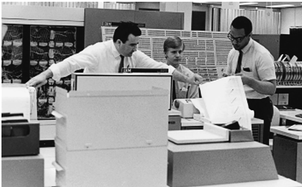
FIGURE E4.17.3 The IBM 360/91 pushed the state of the art in pipe lined execution when it was unveiled in 1966.
